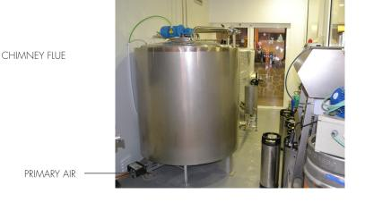
Here, the stew has its sides covered with an insulating material which keeps the temperature and improves the heating times.
